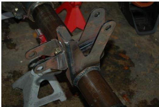
13. Carefully, and with the aid of a helper, remove the differential from under the vehicle and prepare it for final welding of the brackets.
