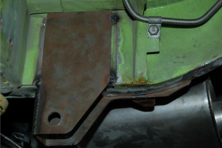
*The picture to the left shows the forward frame bracket on the outside of the rail, firmly against the sheet metal lip of the forward leaf spring mount. Do this on both sides then measure each brackets distance from a fixed point on each side of the chassis. Make fine adjustments to ensure they are positioned at equal distances and square.*
