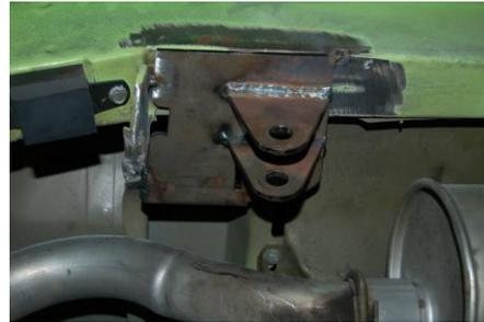
11. Place the left and right upper coil over brackets into position as shown in the pictures above. Carefully tack weld the parts into place by placing tack welds where you can get to them should you need to shift bracket position. Again, double check before placing the tack welds. It is better to get it right the first time, even if it takes longer to do.
