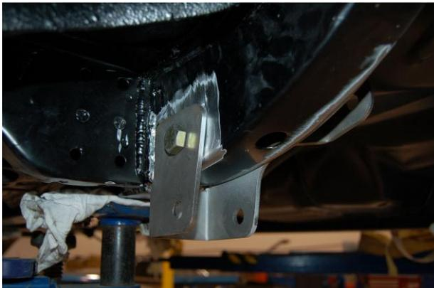
*The measurement to the lower trailing arm hole center should be 55.5". Make fine adjustments to ensure both brackets are positioned at equal distances and square. You can now tack weld these brackets into position.*
