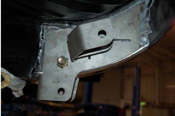
*The pictures to the left show the forward frame bracket on the inside and outside of the rail, firmly against the sheet metal lip.*
