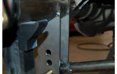
10. Place the upper trailing arm differential brackets into position on the top of the differential tubes. You can see the position by viewing the CAD drawing on page 3. Just like on the lower brackets, tack the upper brackets into position ensuring they are parallel with the lower trailing arms and perpendicular to the differential axle tubes. Place a few tack welds into the corners of the brackets.
