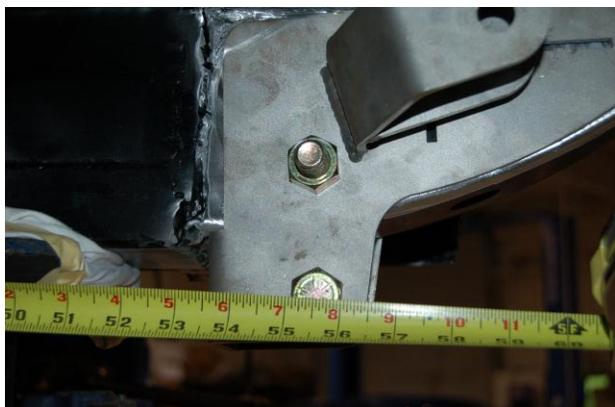
1. Place the forward frame brackets into place. There is a right and left bracket. Correct placement is shown from the inside and outside of the rail in the photos. Make certain the area around the perimeter is cleaned to bare metal allowing a good welding surface. The forward edge of the brackets should be perpendicular to the chassis.
