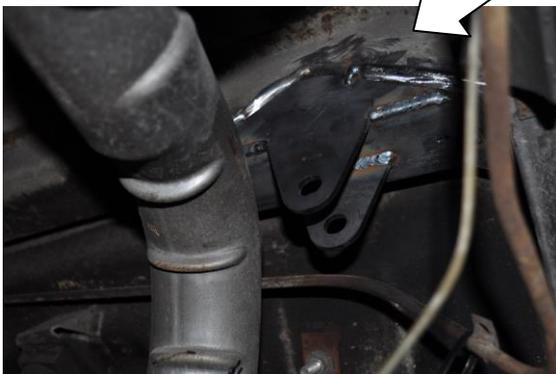
5. Attach the upper and lower trailing arms to the forward frame brackets and hand tighten the nuts onto the bolts. Make certain the upper trailing arms are adjusted to the same length, with about three threads showing behind the jam nut. Do the same for the lower trailing arms.
