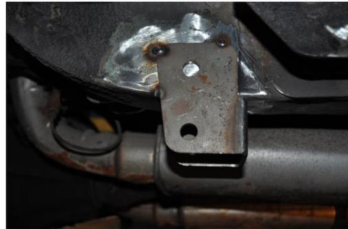
7. Place the assembled trailing arms, with brackets attached, onto the differential. This dictates where the brackets should be. Once again, check the centering of the differential unit and the pinion angle. When it is all correct, tack weld all of the brackets into position.
