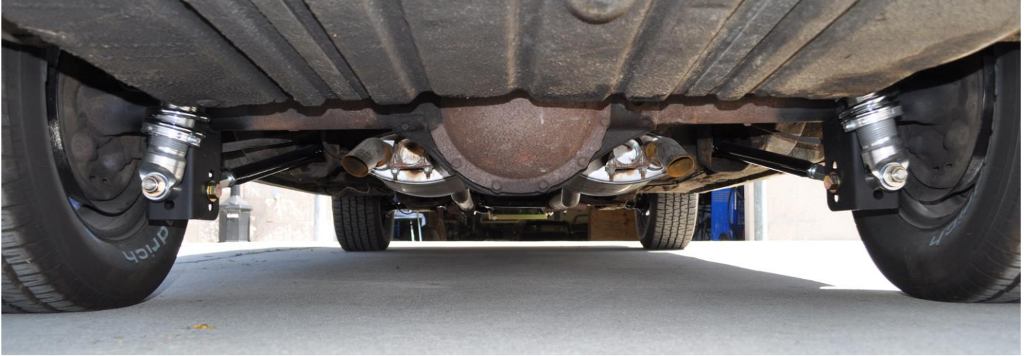
Rebel 4-Link Rear Suspension System (RS-1450)
