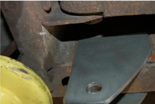
The picture to the right is the inside of the rail. The bracket sits squarely against the parking brake cable clip.
