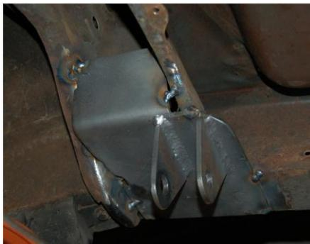
position as shown in the picture to the left. Carefully tack weld the parts into place by placing tack welds where you can get to them should you need to shift bracket position. Again, double check before placing the tack welds. It is better to get it right the first time, even if it takes longer to do.
