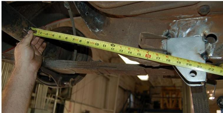
3. Get both upper and lower trailing arms and screw the rod ends in until about three threads are showing between the jam nut and the body of the rod end. Only hand tighten the jam nut. The length of both
