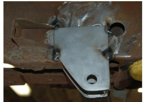
1. Place the forward frame brackets into place. There is a right and left bracket. Correct placement is shown from the inside of the rail and the outside of the rail in the photos below. Make certain the area around the perimeter is cleaned to bare metal allowing a good welding surface. The forward edge of the brackets should be perpendicular to the chassis.
